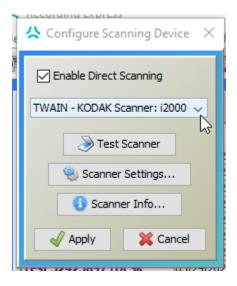
If your Test Scanner image comes back a little off you can change the Scanner Settings. Typically the default is just right.
